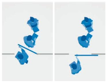
Figure 4. Sliding door reduces the risk of collision
