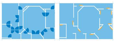
**Figure 3.** Sliding vs swing doors can save up to 15 % of space based on opening area that swing door requires
