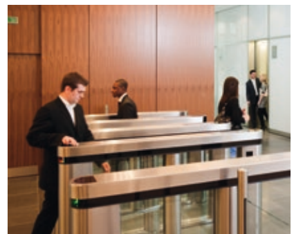
The access control system can activate guided transport operation to the KONE Destination Control System (DCS) when the user passes through
