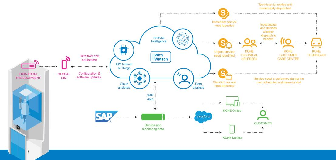
Information on the key operating parameters, usage statistics and faults is sent in real time to KONE's cloud service, where the analytics are located.
